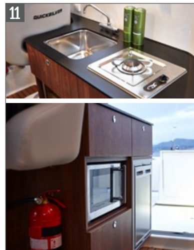
Galley with sink & tab with refrigerator, single burner stove and microwave
