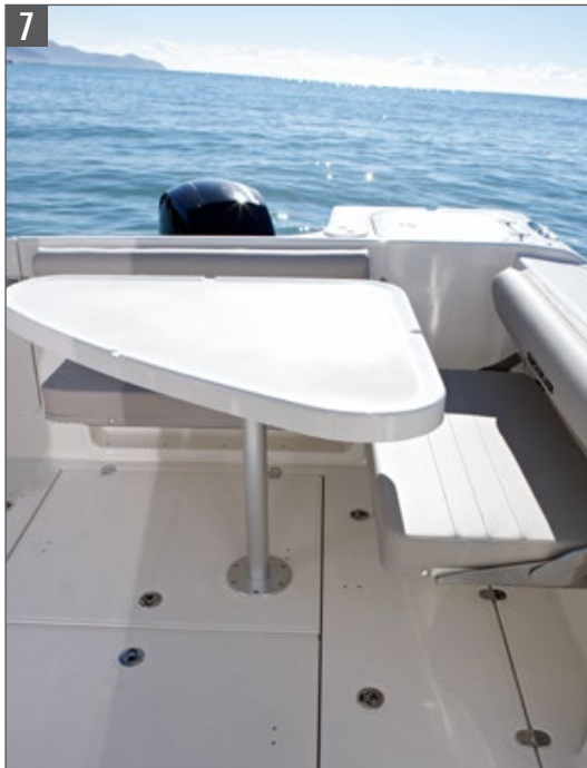
Aft & port flip down bench seats and cockpit table as part of Cockpit Comfort Pack
