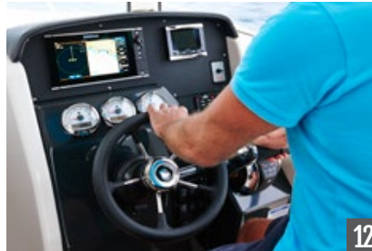
Helm with hydraulic steering, SmartCraft, 9" GPS/Chart plotter, stereo and 12v outlet
