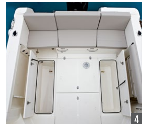
2 fish lockers with standard drains
