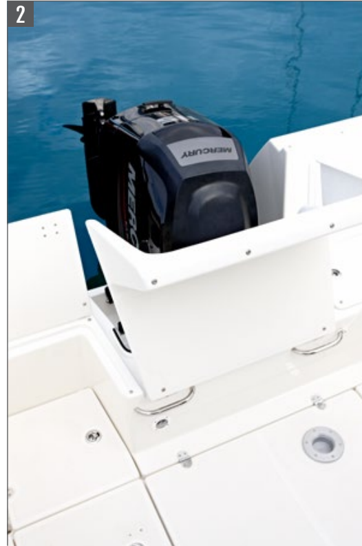
Folding seat allowing full engine tilt position
